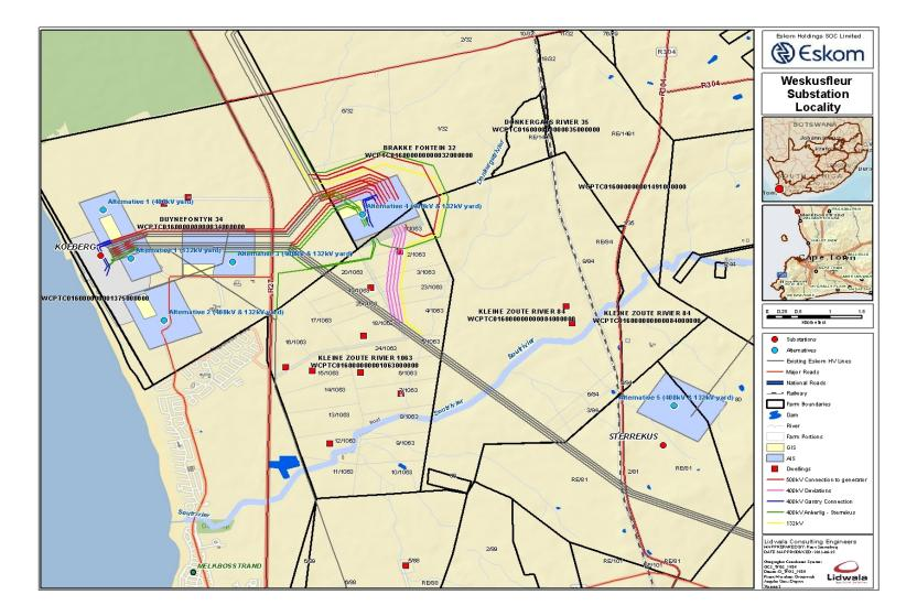
**Figure 4.8**: Locality map showing the proposed turn in including additional line arrangements for alternative 4 (Note that the extent of the AIS on the map is larger than required at  $950 \times 750$  m, the actual required size is  $760 \times 550$  m)
