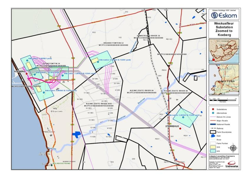
**Figure 4.7**: Locality map indicating all the alternatives (Note that the extent of the AIS on the map is larger than required at 950 x 750 m, the actual required size is 760 x 550 m)
